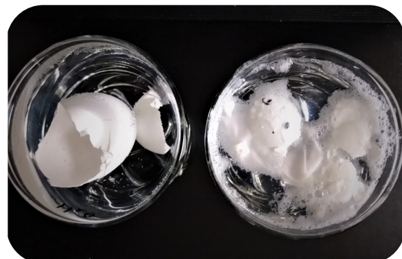
Egg shells in water on the left and in vinegar on the right after 24 hours.
