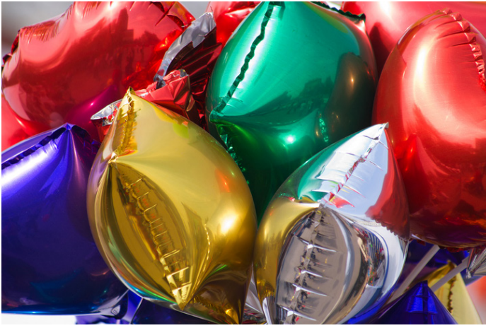
Mylar balloons get their shine from a coating of aluminum (Source: psam via Getty Images).
