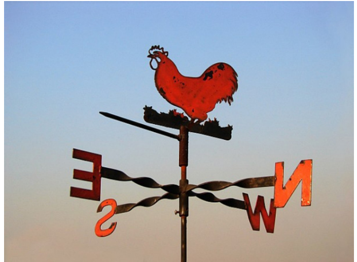
Weather vanes show the direction that wind comes from (Source: Nevit Dilmen [CC SA 3.0] via Wikimedia Commons).
