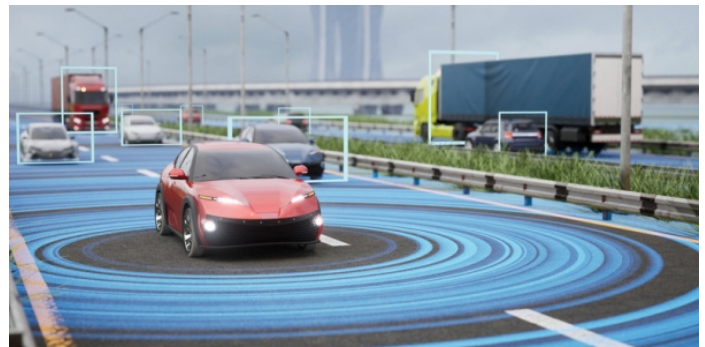
3D image of self-driving cars. The rectangles show where the car detects other vehicles (Source: 3alexnd via iStockphoto).
