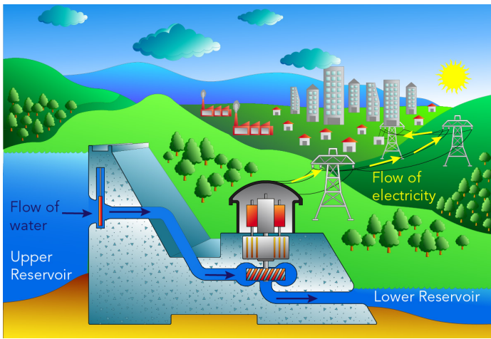
Pump storage in the daytime (Let's Talk Science using an image by bubblea via Getty Images).
